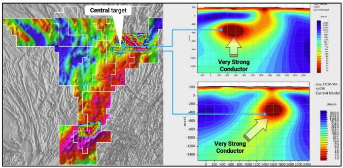
Figure 3: Central AMT anomalies (low resistivity, high conductivity), as announced on 16 March 2022
