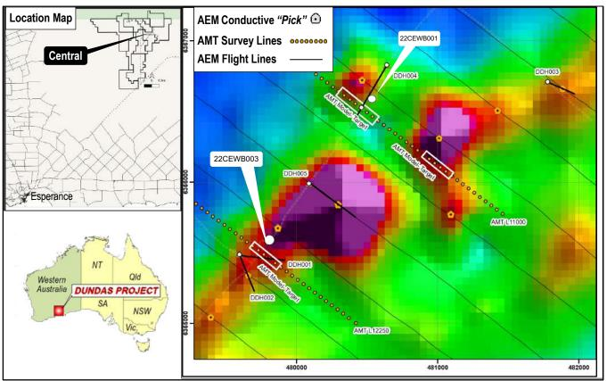
Figure 2: Late-time (B Field channel 41), aerial electromagnetic (AEM) anomaly trend at Central target with AMT model drill targets in white boxes (lines 12250 and lines 11000) and locations of planned drill holes DDH001 to DDH005 marked.
