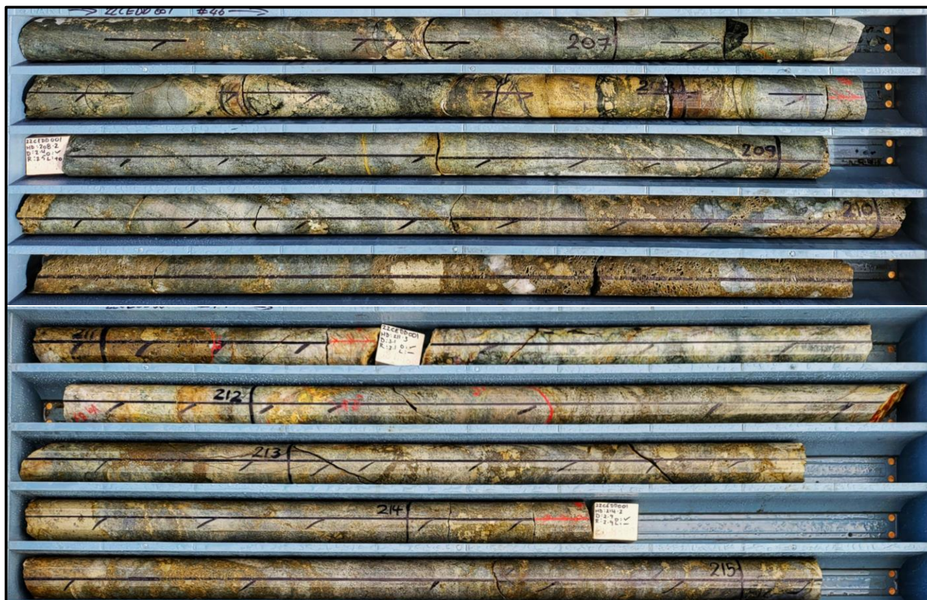
Figure 8: 22CEDD001 drill core 208.2m-215m, massive and highly disseminated sulphides (predominantly pyrite)
