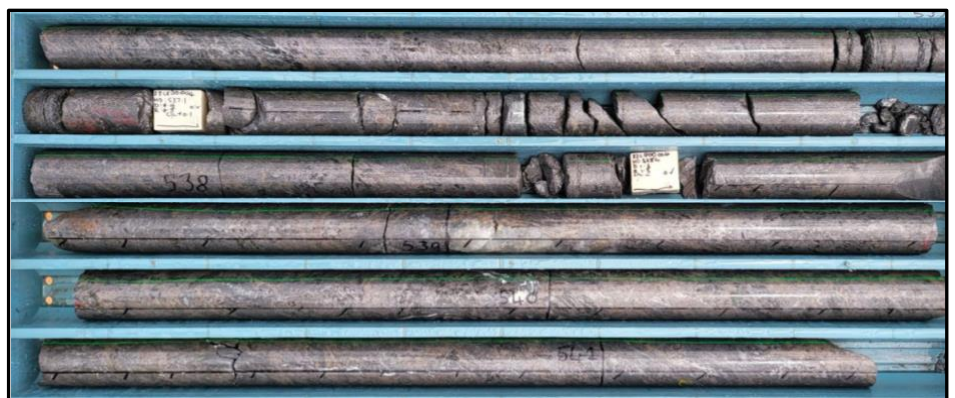
Figure 1: Drill core (22CEDD004) ~536m to 541.4m. Semi-massive pyrrhotite, disseminated pyrite and trace chalcopyrite.
